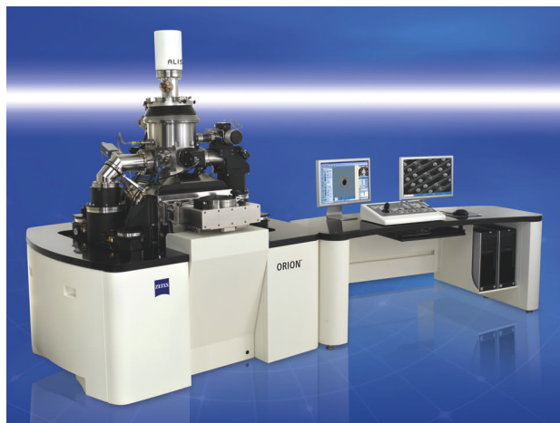
The Zeiss Orion microscope uses a stream of helium ions rather than electrons to generate signals. Helium-ion microscopy offers spatial resolution of 0.2 nm. Courtesy of Carl Zeiss SMT.
