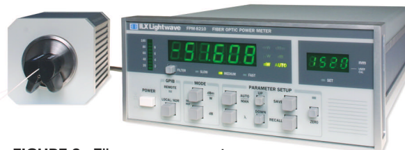
FIGURE 3. Fibers can connect directly to FO power meters and FO test heads.
